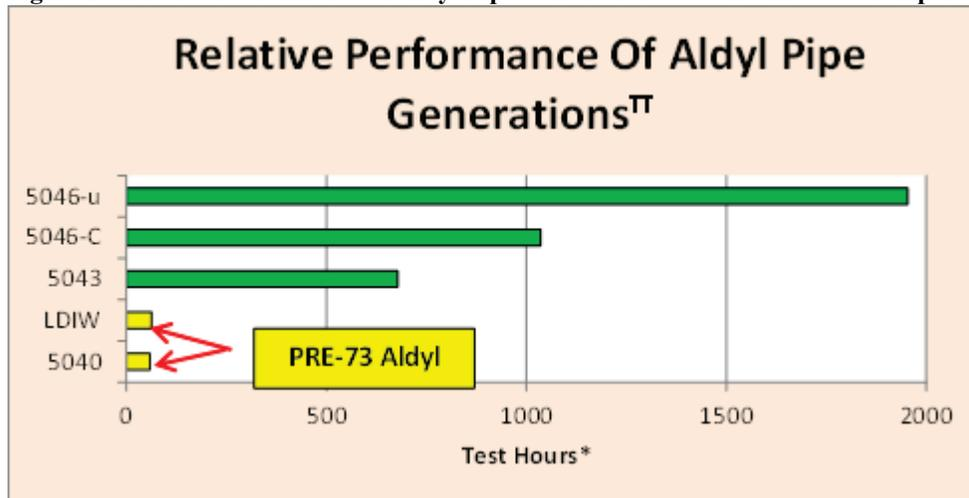
Note: <sup>TT</sup>Based on testing at single condition. For more detailed performance characterizations see section on Performance Comparison of Aldyl Materials. \*Testing conducted at 80°C on 2" Pipe at nominal test stresses of 450-470 psi with Water internal/Water external. All failures were SCG failures initiating at the inner pipe bore.
